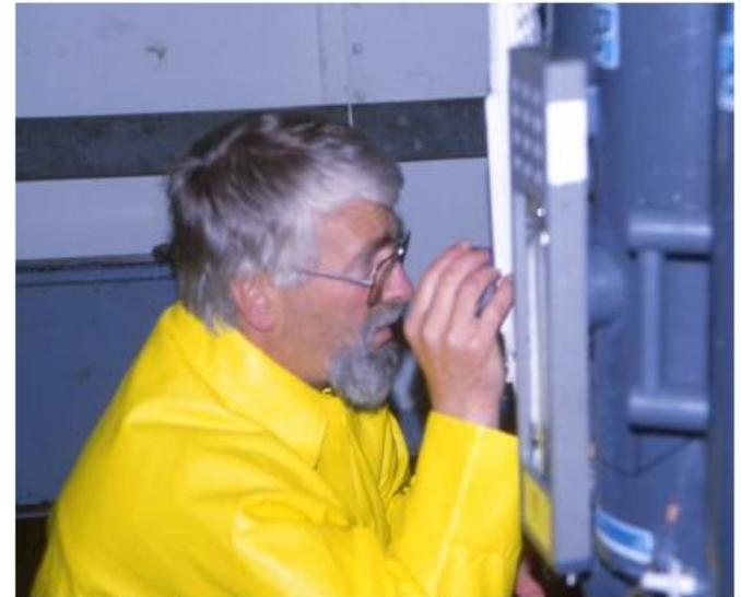
Fig. 6.22. Reading reversing thermometers
