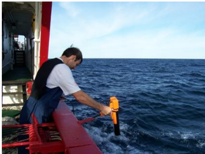
FIGURE S16.18 An expendable bathythermograph (XBT). Source: From NOAA UOTC (2009).
