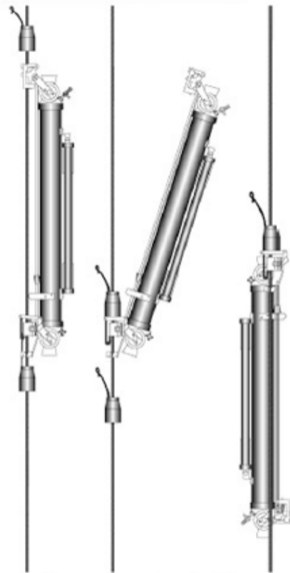
Nansen water bottles before (I), during (II), and after (III) reversing. (From Dietrich et al. 1980)
