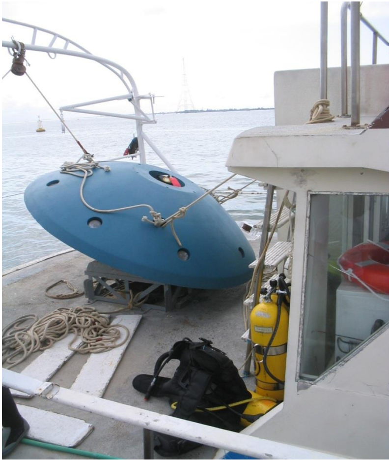
ADP - Acoustic Doppler Current Profiler
